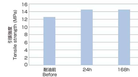
試験油/Test Oil : ASTM IRM902
