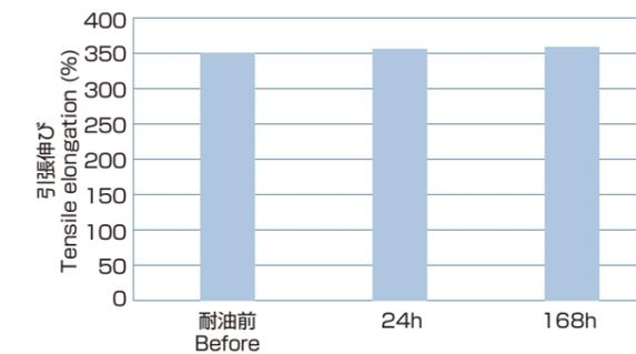
試験油/Test Oil : ASTM IRM902
