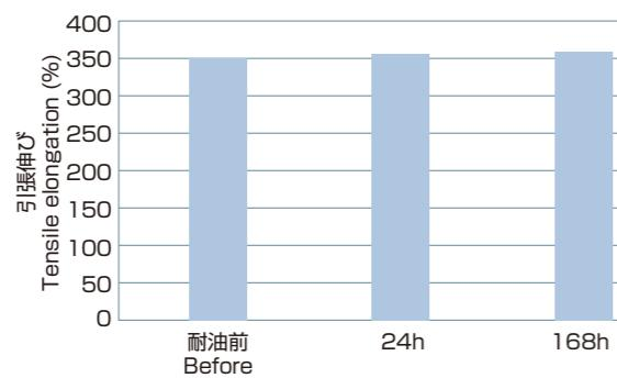
試験油/Test Oil : ASTM IRM902
