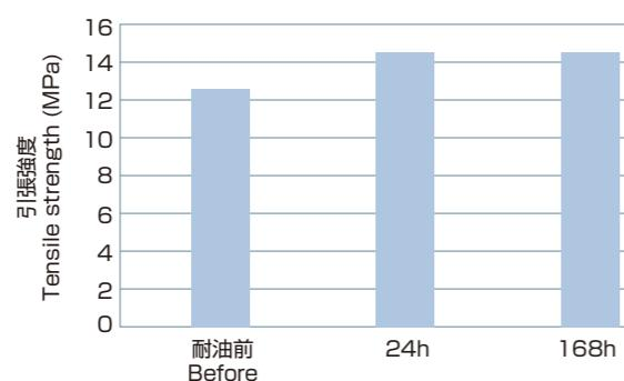
試験油/Test Oil : ASTM IRM902
